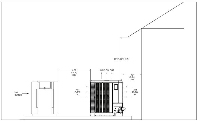
Figure 2. Installation Clearances
