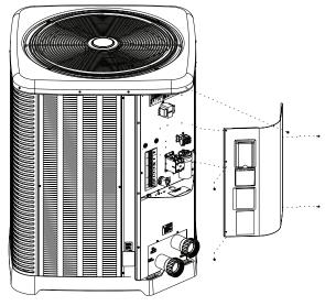
Figure 11. Sheet Metal Screws to Remove Control Panel
