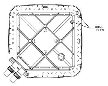
Figure 10. Condensate Drain Hole Locations
