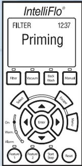
The Priming settings determine how long IntelliFlo VF will try to prime before it reports an error. This is a critical setting for proper operation. The lower the time setting, the quicker a priming error is reported if the system is difficult to prime.
