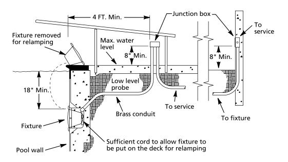
Figure 1 – Lamp Housing Installation
