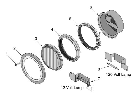
Figure 2 - Replacement Parts Sunbrite™ Lamps Exploded View
