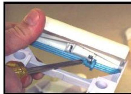
2. Remove the front and rear flaps from the cleaner by inserting a small flathead screwdriver between the flap and the lower body near the pivot points. See Figures 27 & 28.
