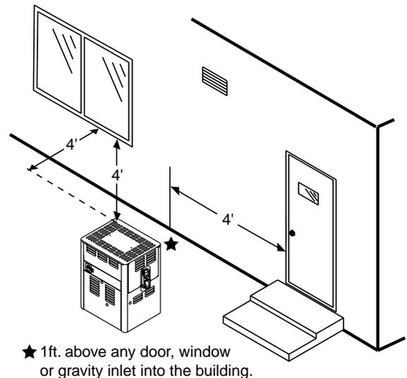
★ 1ft. above any door, window or gravity inlet into the building.
