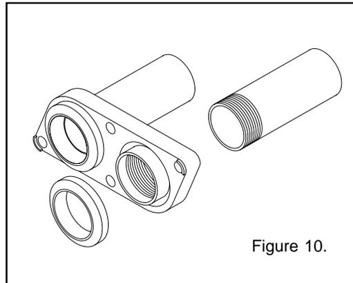
1. Insert 2 in. rubber gaskets over 2 in. gasket retainer rings molded to bottom of Quick-Flange II; see Figure 10.
