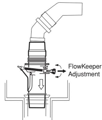
**Install the FlowKeeper Valve with the arrow facing down towards the skimmer pipe.**
