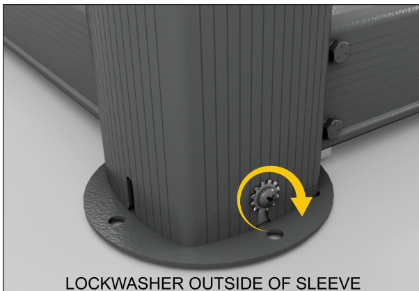
FIGURE 20: TIGHTEN SCREW ON EACH SLEEVE
