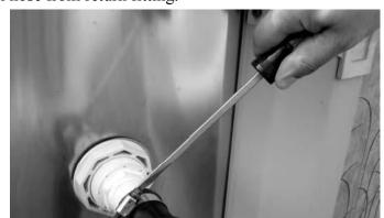
7. Take the hose end removed from pool return and connect to hose adaptor attached to the header. Tighten hose clamp with screwdriver.
