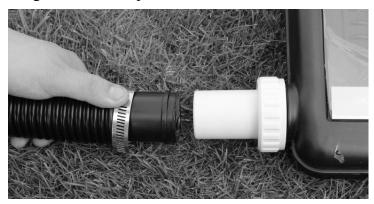
8. Connect provided flex hose to the end labeled "To Pool" and the opposite end to the return fitting. Tighten hose clamp with screwdriver.
